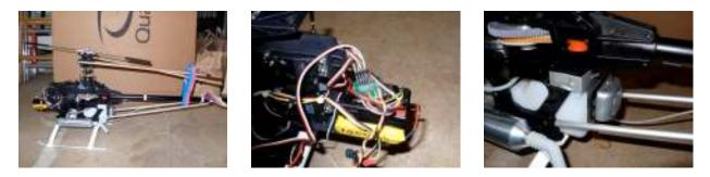
The Raptor - The close-up on the front show the Rx and the circuit board "brain" of the HeliCommand on top of the Rx. The close-up of the rear shows the gray gyro/optical sensor attached to the back of the fuel tank.
