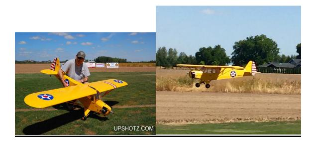
106" Wingspan68" Long Zenoah G26 Power (Magneto Ignition) Hitec Servo's Aero works Operating Beacon Light Articulating Gear NiMH Batteries Smart Fly Kill Switch
