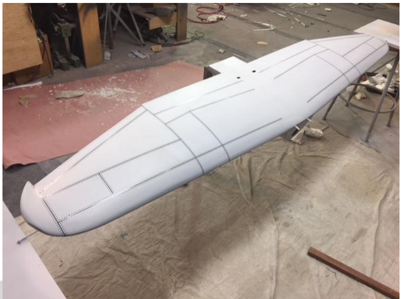
P-47 Wing, Rivets and Panel Lines Ready to Prime
