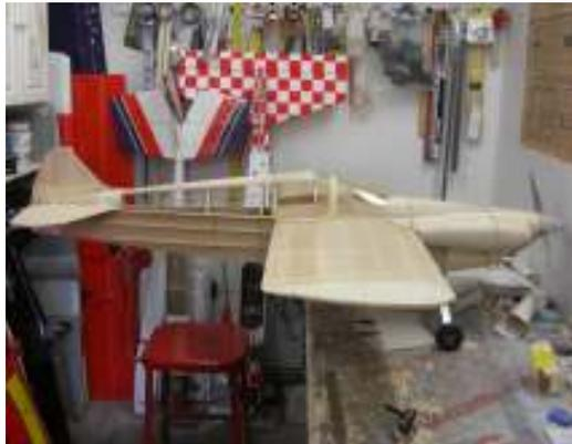
Bonzo is coming along!! I did a weight and balance check ( CG ). And not to bad. I will have to add weight to the tail, Install 3 servos in the tail and place the battery at the trailing edge of the wing. all normal stuff..
